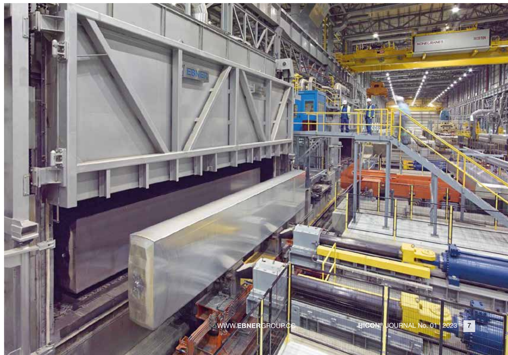
EBNER pusher furnace (furnace entry) with an extremely long rolling ingot in a state-of-the-art plant
